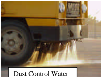
Dust Control Water
